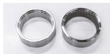
(Left) Component before broaching (Right) Component after broaching
